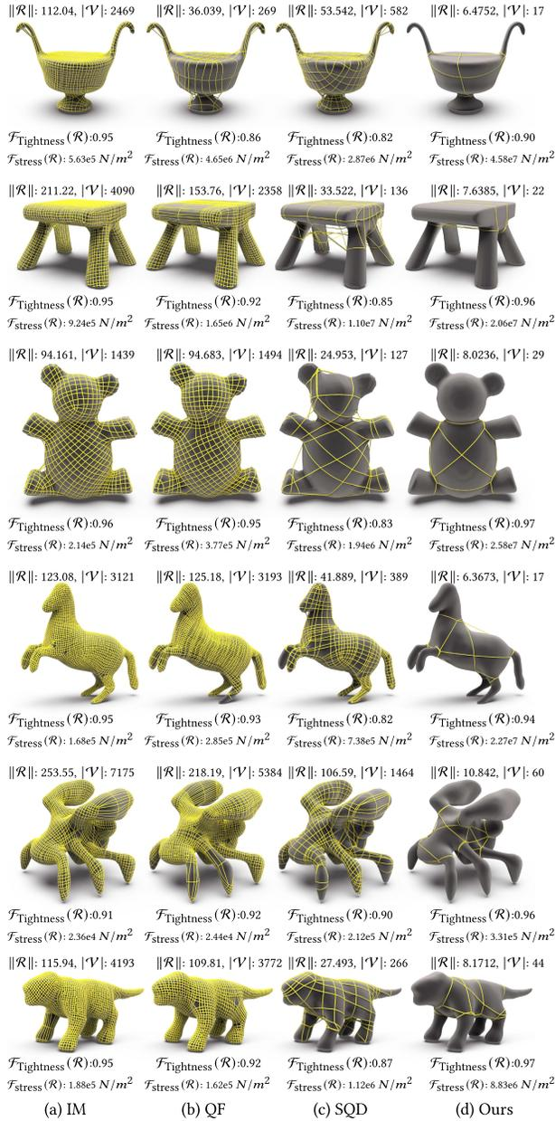
Fig. 24. Comparing with the dual layout-based rope net. The final rope nets (a–c) are initialized by IM [Jakob et al. 2015], QF [Huang et al. 2018], and SQD [Tarini et al. 2011a] and tightened using our tightening algorithm.
