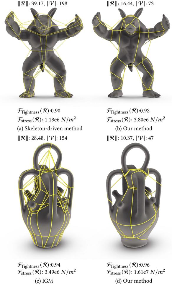
Fig. 25. Comparison on the models with sharp feature and high genus. The rope nets (left column) are the results of the Skeleton-driven method [Usai et al. 2015] and IGM method [Bommes et al. 2013a] taken as initializers and tightened by our tightening algorithm. The rope nets (right column) are our results.
