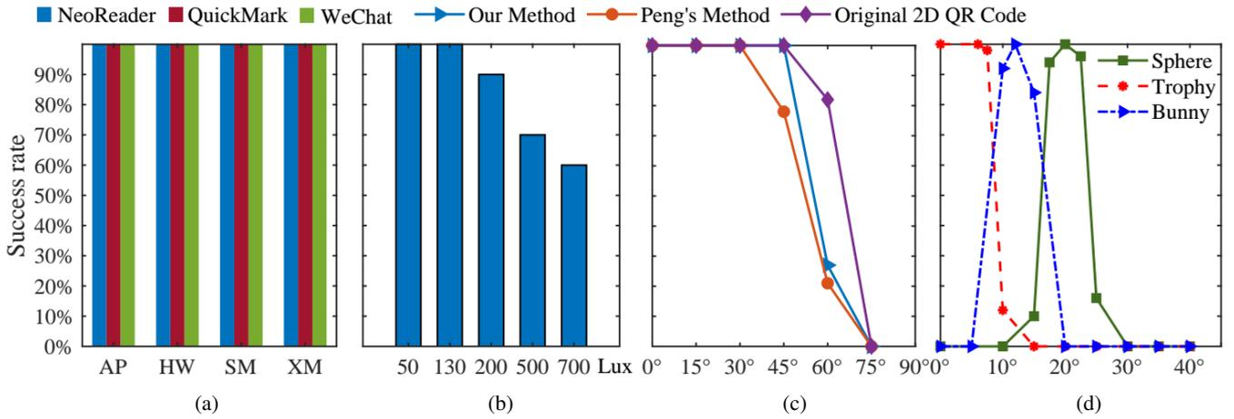
**Figure 18:** Robustness of our 3D-QR-codes in terms of different decoders and mobile phones (a), different lighting environments (b), different scanning angles (c) and different directional light angles (d). AP, HW, SM, XM denote iPhone, Huawei, Samsung and Xiaomi mobile phones, respectively.
