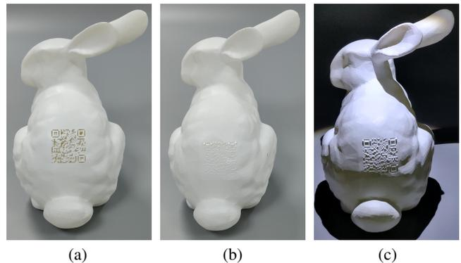
**Figure 1:** 3D-QR-code carvings on bunny’s back. In (a) code is carved by [PLL\*19] under ambient light. Our method generates unobtrusive codes under ambient light in (b), yet readable under directional light in (c).
