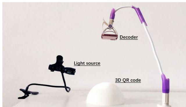
**Figure 17:** Environment setup consists of a spotlight, a standard QR decoder and the 3D printed model with its optimized 3D-QR-code.
