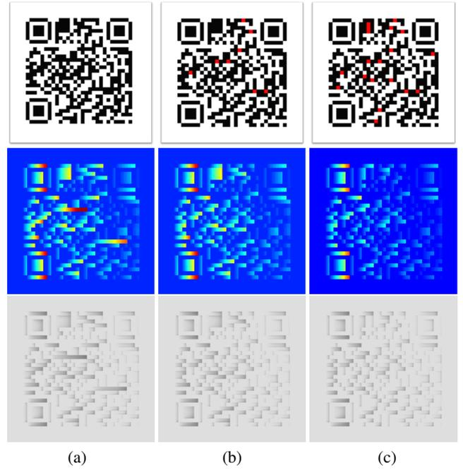
**Figure 9:** Module optimization. Columns (a-c) are initial, mid, and final black module flipping, respectively. Rows, top to bottom, are the QR image (flipped modules in red), the corresponding depth map, and the ambient QR image  $Q_a$ . Flipped QRs are still robust to decoding while consisting of fewer carving modulations.
