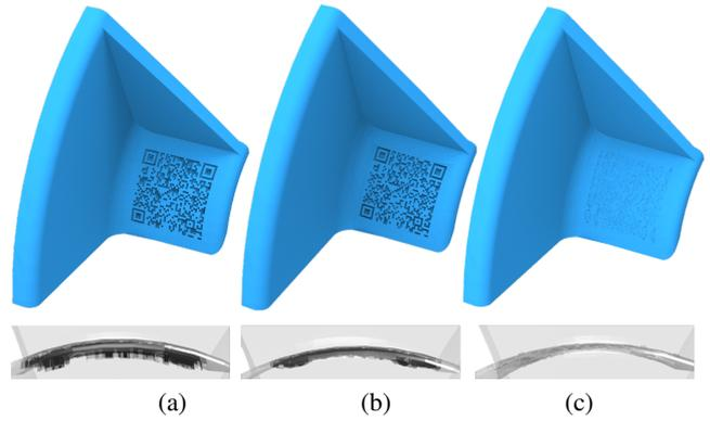
**Figure 23:** Comparison of 3D-QR-code carving on a flange model using the method of [KYJ\*18] (a), [PLL\*19] (b) and ours (c). 1D views on bottom row show carving depths with average depth of 2.18, 1.52, 0.31mm respectively.
