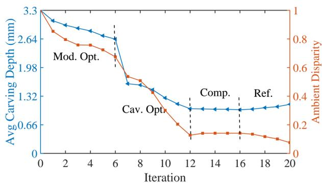
**Figure 16:** Both average carving depth and visual disparity under ambient light decrease along optimization iterations while average carving depth increases in post-processing.
