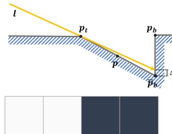
As shown in the left figure,  $\widehat{\mathbf{p}_t \mathbf{p}_b}$  denotes the region of black modules. The initial carving for black modules, i.e.,  $\widehat{\mathbf{p}_t \mathbf{p}_b}$  is determined by the intersection between  $\mathbf{p}_t$  and  $\mathbf{l}$ , which is  $\Delta$  deeper along the projection direction.
