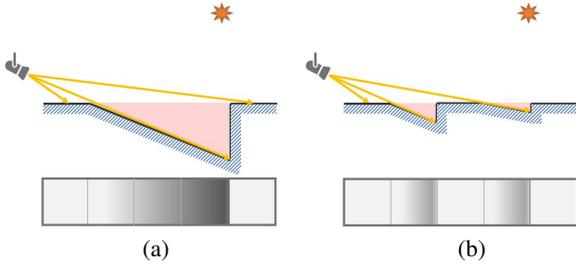
**Figure 7:** Continuity suppression 1D illustration. By suppressing the black modules continuity (a), the carving depth is reduced accordingly and the QR code is less obtrusive under ambient light (b). Bottom row are corresponding ambient image pixels  $Q_a$ .
