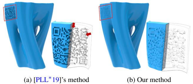
**Figure 24:** Comparison of 3D-QR-code carving on a thin vase model of 2mm thickness between [PLL\*19]'s method (a) and ours (b). Zoom-ins show that the average carving depth (1.74mm) is close to thickness of the vase where the vase is punctured (red arrows) (a), while our result is shallow (0.70mm).
