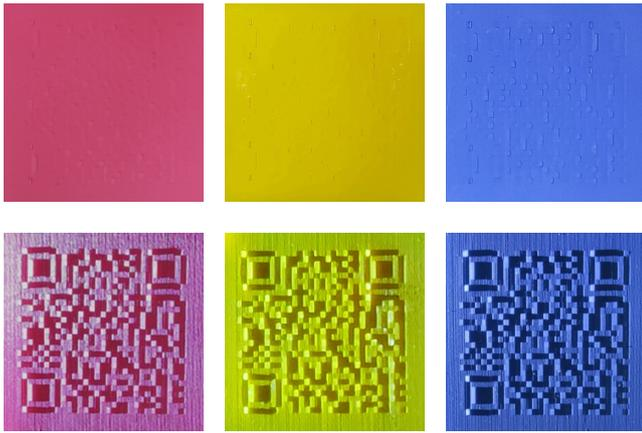
**Figure 21:** A 3D-QR-code printed with different colors under ambient (top) and directional lights (bottom).
