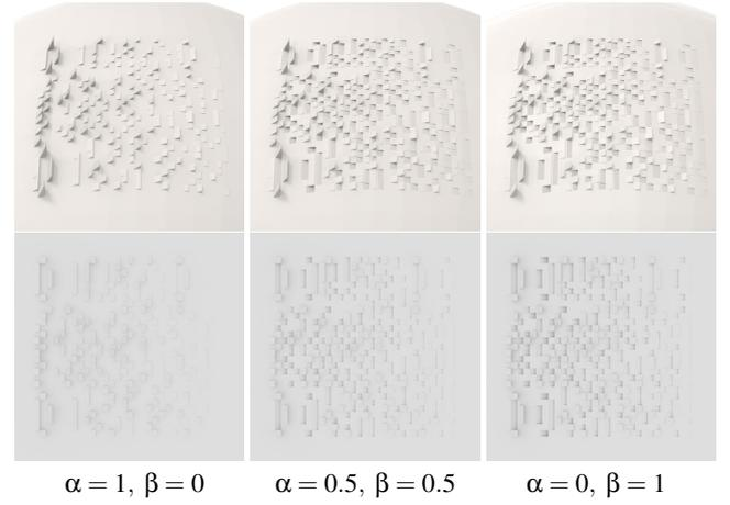
**Figure 15:** Optimized 3D-QR-codes' geometry model (top row) and ambient QR image (bottom row) with different  $\alpha$  and  $\beta$ . The average carving depths are 1.61mm, 1.10mm, and 1.04mm, from left to right. The visual disparities are 1.66%, 2.67%, and 3.44%, respectively.
