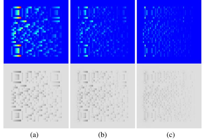
**Figure 12:** An example of carving optimization. Columns (a-c) contain the carving optimization at initial, midway, and final iterations. Rows, top-bottom, are depth map and ambient QR image  $\mathbf{Q}_a$ .
