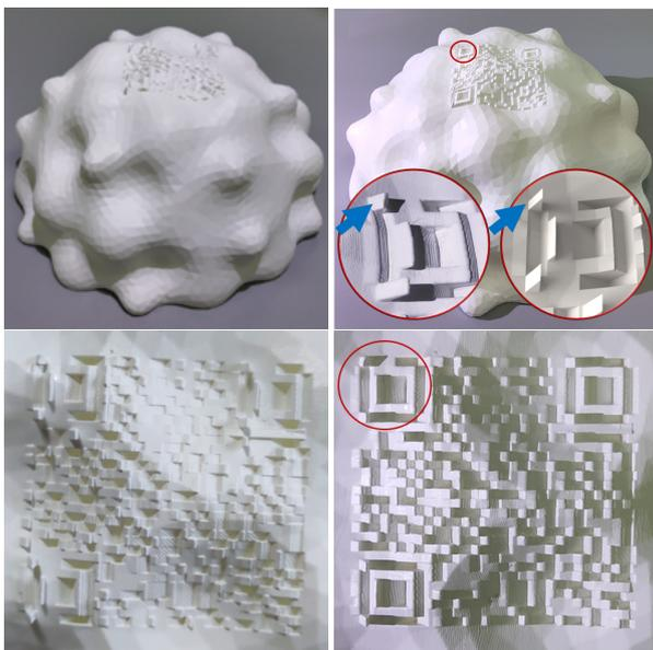
**Figure 26:** 3D-QR-code embedded on a highly bumpy surface. The directional light angle is  $32^\circ$ . The outward carving features circled in red in 3D-QR-code are too sharp and thus unstable.
