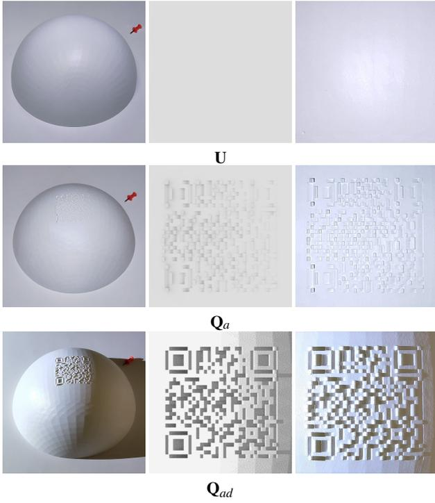
**Figure 6:** 3D-QR-code simulation. Left-to-right columns are the 3D model, simulated image and real photograph. Rows top-bottom depict un-carved model, carved model under ambient light and carved model under both ambient and directional light.
