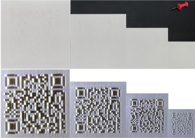
**Figure 19:** 3D-QR-code printed on different region sizes under ambient (top) and directional lights (bottom). Lengths (left-to-right) are 73.8mm, 61.5mm, 49.2mm, 36.9mm.
