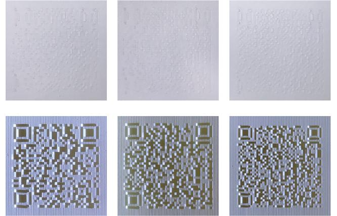
**Figure 20:** Different QR-code versions under ambient (top) and directional lights (bottom) on the same model size (61.5mm). QR version is 4, 5, 6, from left to right, respectively.
