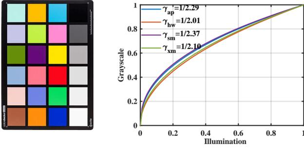
**Figure 5:** Gamma correction curves for gray values and their according illumination value. We photograph the color checker (X-Rite) using mainstream mobile phones such as iPhone(ap), Huawei(hw), Samsung(sm) and Xiaomi(xm) and then test their gamma values using iQstest. The gamma correction curves for the gray values and their according illumination value are plotted in the right figure.
