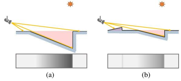
**Figure 8:** Carving modulation 1D illustration. By modulating the carving region (a), the carving depth is reduced accordingly and the QR code is less obtrusive under ambient light (b). Bottom row are corresponding ambient image pixels  $Q_a$ .
