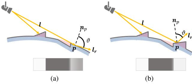
**Figure 13:** Brightness compensation 1D illustration. The white module could be mistaken for the black (a) due to occlusion under the directional light. By modifying the inclination of the white module we compensate the lightness to make it the right color (b).
