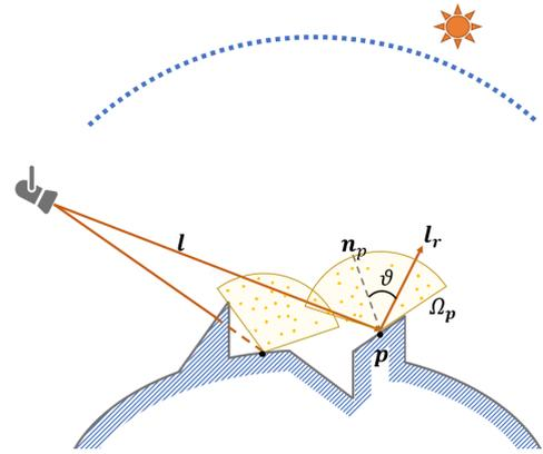
Figure 4: 1D illustration of directional occlusion computation.
