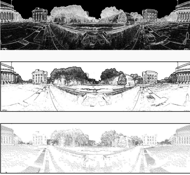
Figure 3: Feature extraction of the panoramic scan shown in color plate Figure 8. From top to bottom: image encoded by the feature degree, the feature points, and dithering points.
