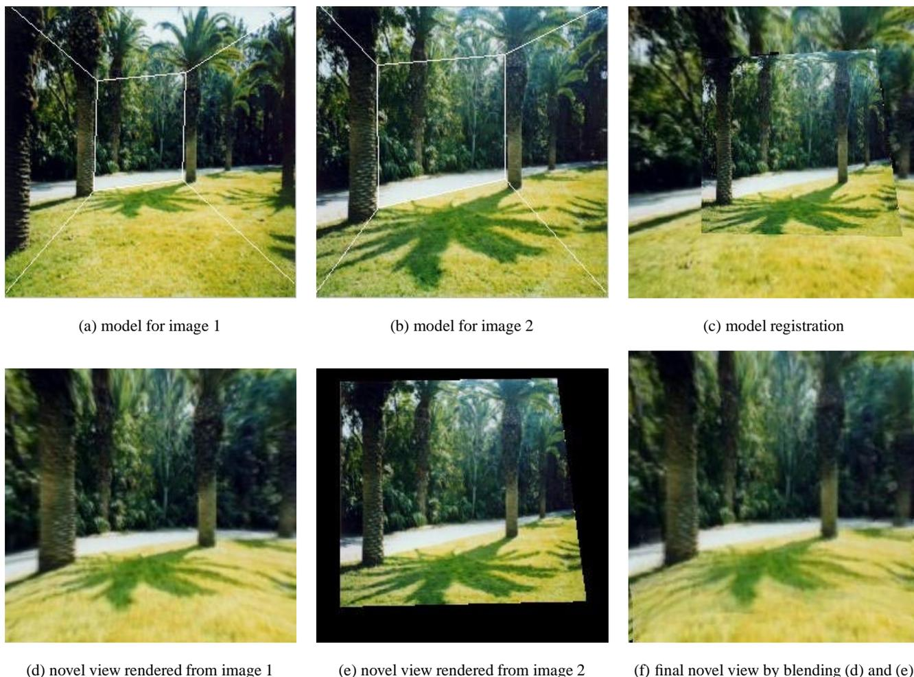
Figure 2: Algorithm Overview. (a) and (b) show the original input images and the models we used; (c) shows the registered models; (d) and (e) show a novel view from each model and (f) shows the final blended images.
