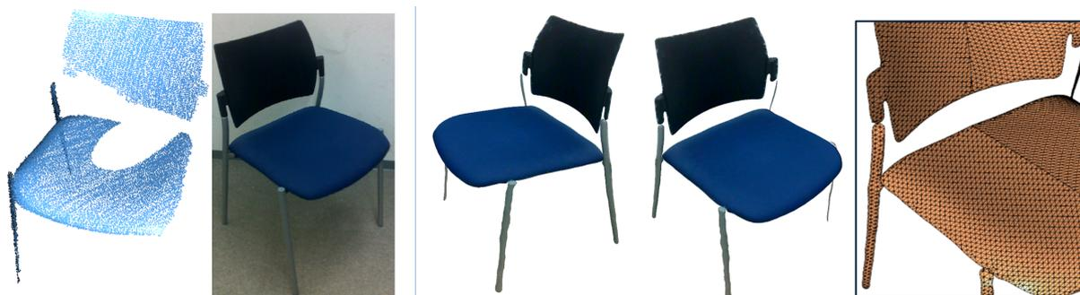
**Figure 1:** Given a partial 3D scan and a 2D photograph (left), we lift 2D shape structures into 3D yielding a faithful textured mesh reconstruction (right).
