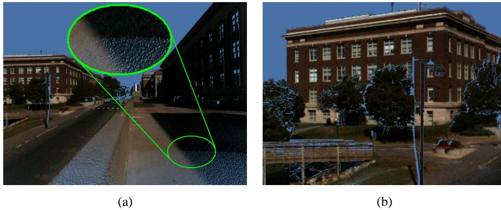
Figure 5: Two novel views of Walter Library and Fraser Hall (1,319,214 points and  $800 \times 600$  image resolution): (a) using averaged 3D point size for each region leads to visible boundary between regions and/or holes (within green circles). The region segmentation on the ground is shown in Figure 2j; (b) a close-up view of Fraser Hall (segmented in Figure 2(a-h)).
