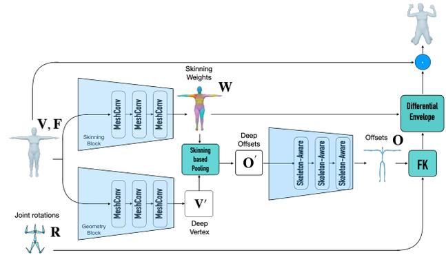
Fig. 3. The envelope deformation branch. Given a mesh in T-pose ( $\mathbf{V}, \mathbf{F}$ ) and joint rotations ( $\mathbf{R}$ ), our network infers the skinning ( $\mathbf{W}$ ) and rigging ( $\mathbf{O}$ ) parameters via indirect supervision by observing the articulated character vertex positions.
