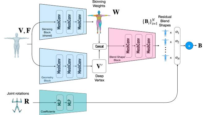
Fig. 4. The residual deformation branch predicts blend shapes and blending coefficients based on the input mesh connectivity and input joint rotations. The network learns to estimate blend shapes for arbitrary mesh connectivities and blending coefficients that are conditioned on the joint rotations.
