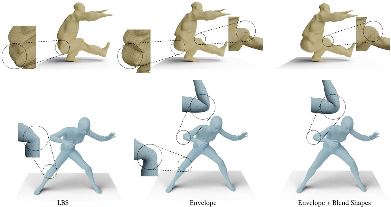
Fig. 7. Our predicted envelope deformation produces favorable results, compared to LBS. Adding neural blend shapes to the enveloping results in corrective pose-dependent displacement, which improves the deformation quality in the joint regions.
