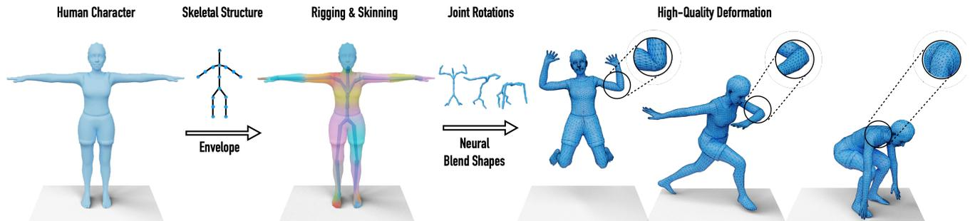
Fig. 1. Our neural skeletal articulation network learns to rig and skin an input character with arbitrary connectivity, and generates neural blend shapes. Our framework produces pose-dependent displacements that result in high quality deformations, especially in the joint regions.
