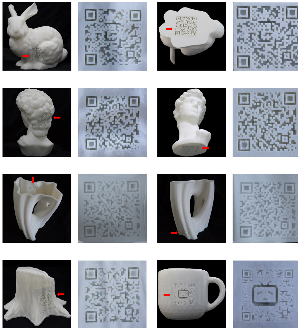
Fig. 17. The printed 3D-QR-codes on arbitrary shapes, and the zoom-ins of the QR codes.
