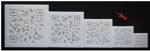
Fig. 12. A 3D QR code printed in different sizes. The length is 73.8 mm, 61.5 mm, 49.2 mm, 36.9 mm, 24.6 mm, respectively, from left to right.
