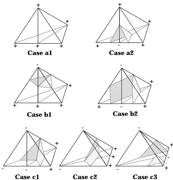
Figure 4: Isosurface configurations after subdivision of the three cases in Fig. 3
