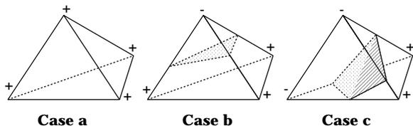
Figure 3: Isosurface configurations within a tetrahedron
