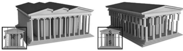
Figure 14: Results showing certain limitations of our method. Left: unnatural partitioning (bottom-left insert) of the input results in unnatural retargeting results. Right: aligning only the bounding boxes but not edge features in the structural elements can result in visible artifacts; bottom-left insert shows the partitioning used.
